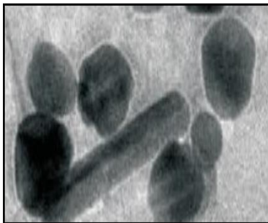
Figure 1: TEM Image of Prepared AgO Nanoparticles with 100 nm Magnification
